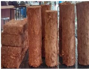
Image Showing the Sample Preparation for Strength Tests
