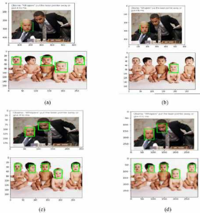
Figure 8.7 Outputs of Different Face Detection Algorithms: (a) Face Detection using Haar Cascade (b) Face Detection using LBP Cascade (c) Face Detection using MTCNN (d) Face Detection using SSD
